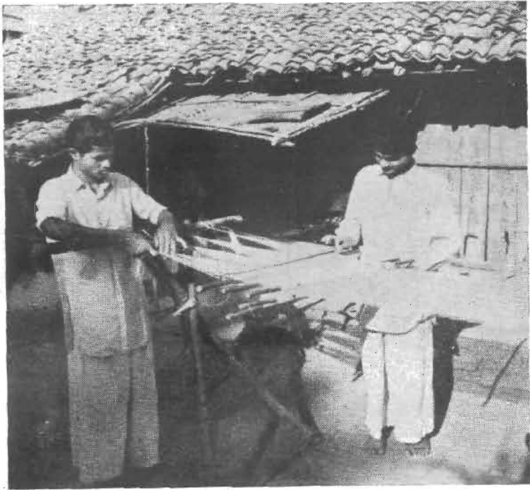
Cleaning of stretched warp.
