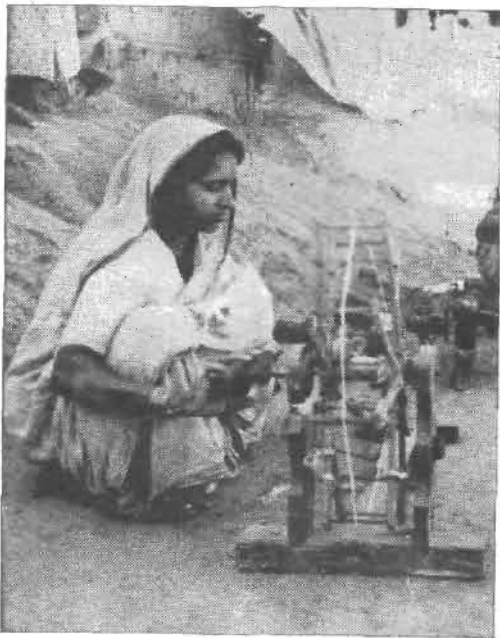
Winding the Kosa yarn on bobbins.
