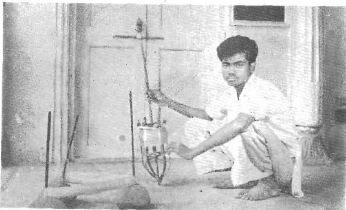
The weft yarn is transferred from "Kupe" to the "Parti"
