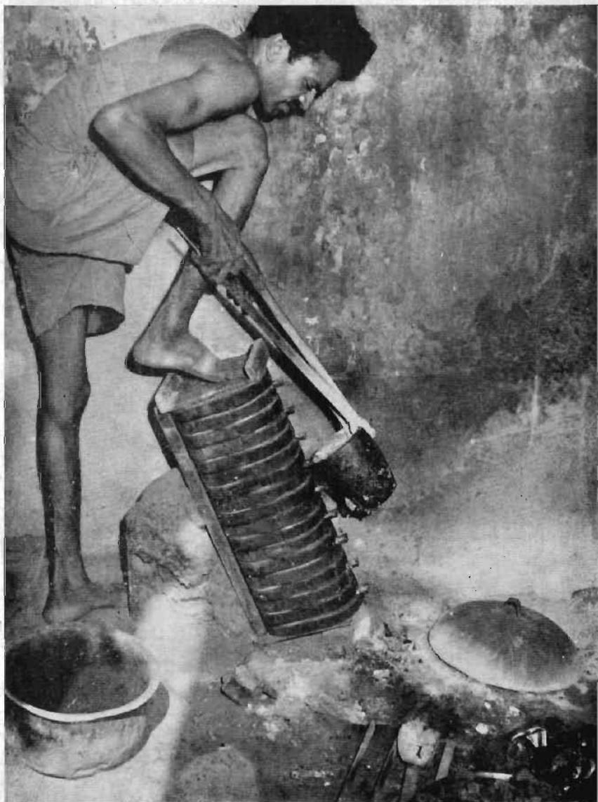
*Moulds arranged in series fed with liquid metal*
