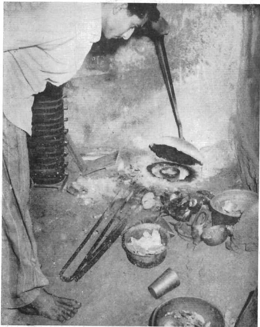
*Melting brass scrap in a furnace*
