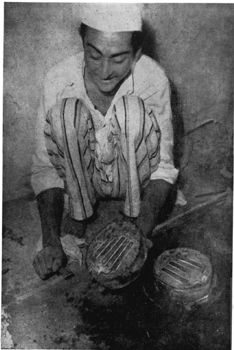
*Upper and lower parts of the mould*
