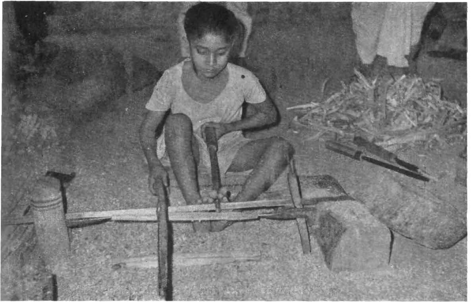
Working on 'Sangheda'—a hand-operated lathe.
