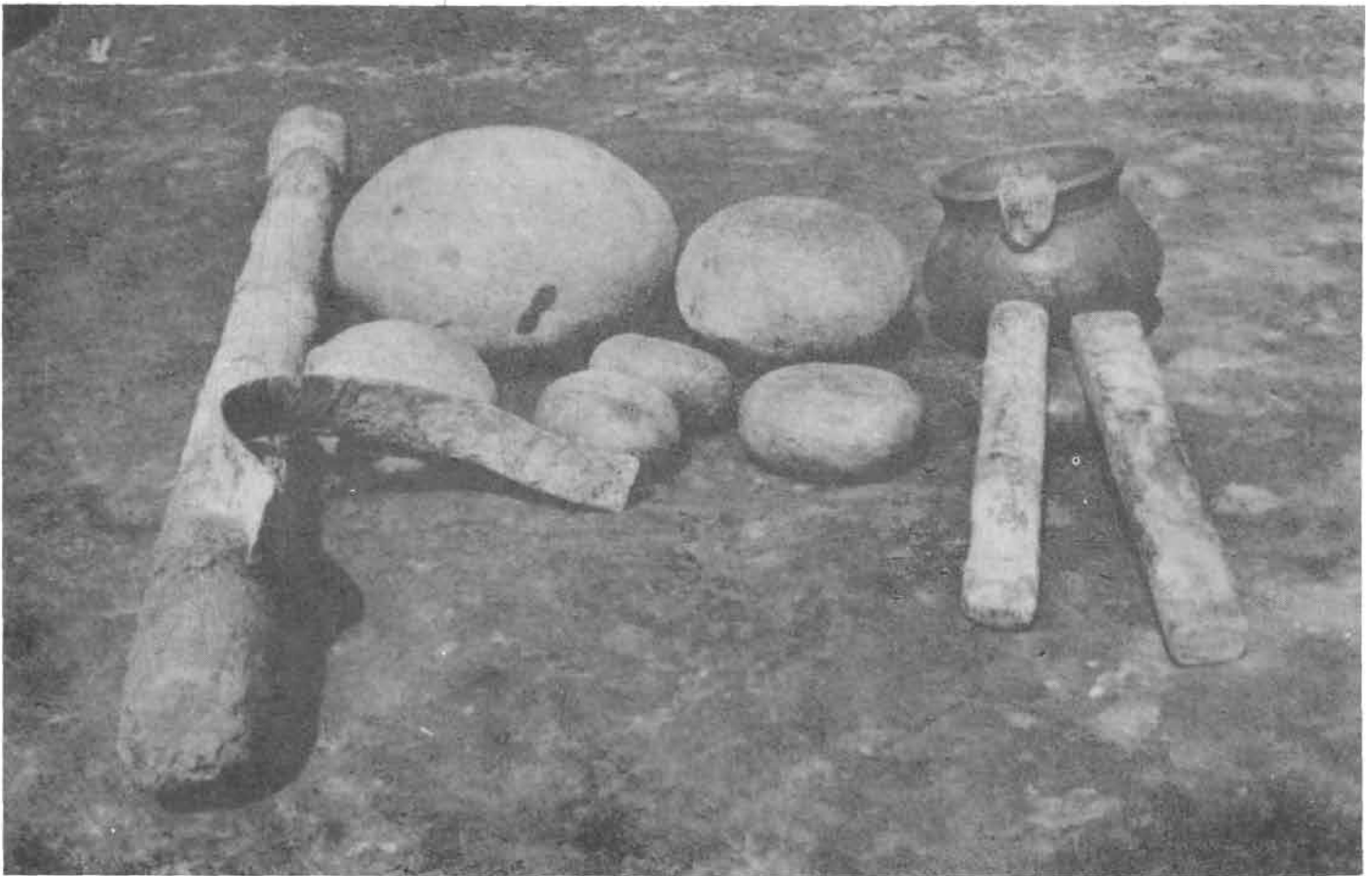
A few tools and implements : Clock-wise from behind—Stones of different size, small earthen vessel for storing water and a piece of cloth constantly used in every stage of products, mallets, 'Kortara'—a culler made of tin for cutting clay in initial stage and 'Gajanbari' or pestle used in kneading the clay. .
