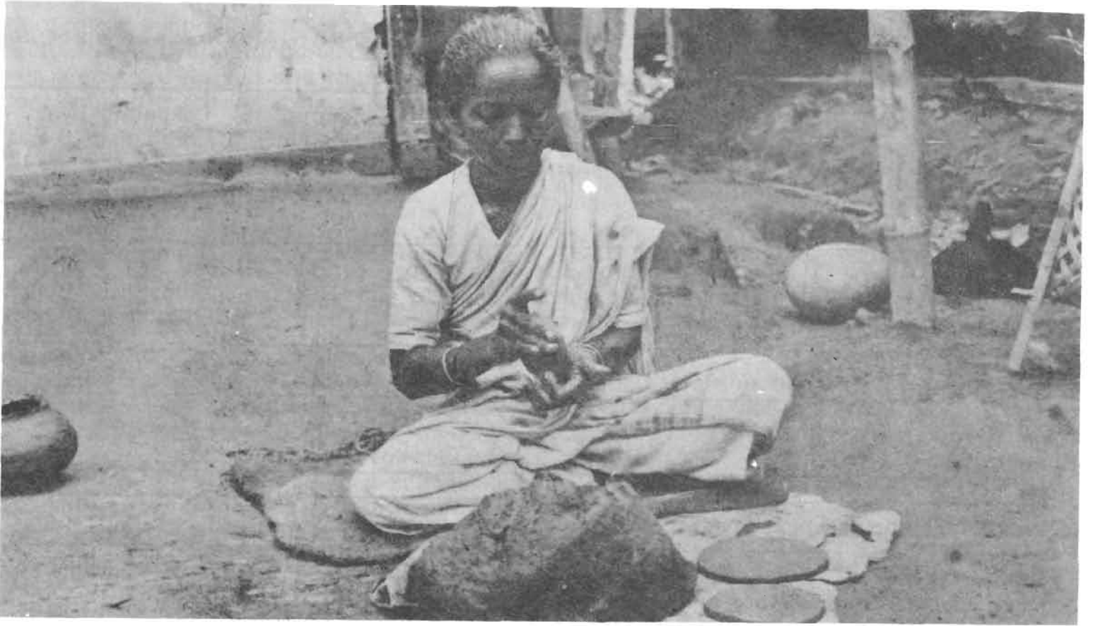
First step in production : Making of 'Don'—a flat and circular structure of clay
