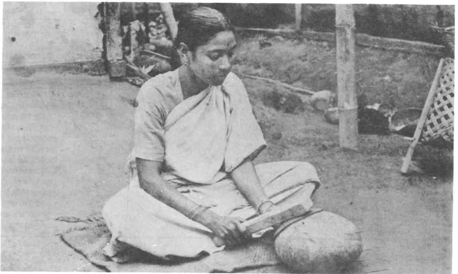
Second step : Beating the 'Don' with a mallet into the shape of a cap
