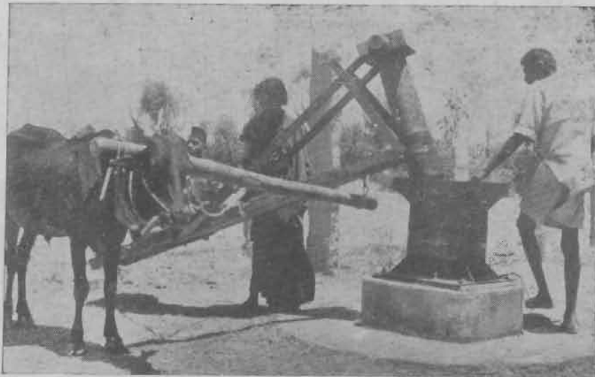
10. An improved Hubli-type wooden oil extractor. Note that a single bullock can work an extractor of this type
